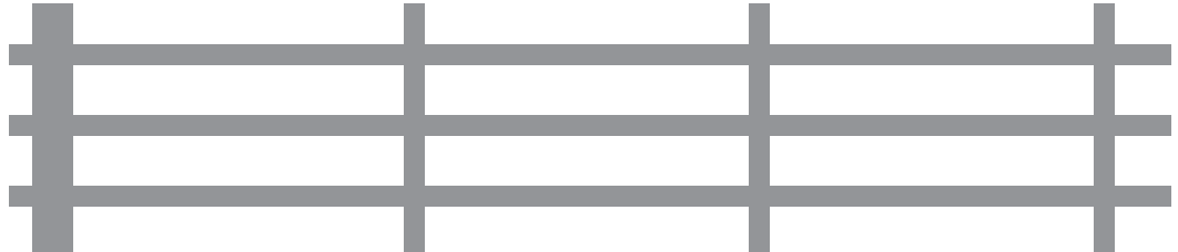
MAX-FLOW 68% OPEN SLOTS 1/4" X 1-1/2", IN ROWS ACROSS WIDTH OF SHEET. VERTICAL BARS 3/32" WIDE, WITH EVERY THIRD BAR 3/16"
